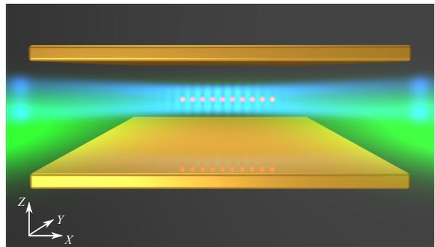
Circular Rydberg atoms are trapped in a blue-detuned dipole trap inside a spontaneous-emission inhibiting structure. We aim at the realisation of quantum simulations with tens of atoms during several tens of seconds.
