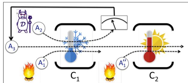
Two high-quality superconducting cavities  $C_1$  and  $C_2$  store microwave field for several tens of microseconds. Circular Rydberg atoms  $A$  cross the cavities one-by-one. Precise real-time control of their interaction with the cavity fields allows us to realize different thermodynamical components, like reservoirs, batteries, Maxwell's daemon, etc. and perform on them heat transfer and work.
