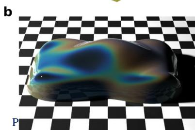
Part of a macroscopic object covered by a disordered metasurface specifically designed. **a.** Sketch of the metasurface. **b.** Appearance obtained by our nano-rendering tool. The appearance of the object drastically changes when moving around the object or changing the light source position.
